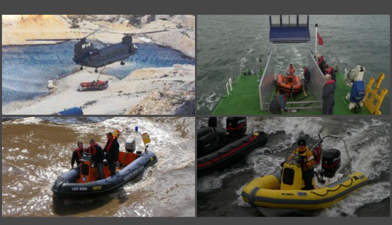
The highly popular Assault Series designed with our performance deep 'V' hull is one of a kind, producing outstanding acceleration and handling characteristics. With large buoyancy tubes offering maximum safety and stability, the Assault series is perfect for rescue organisations and light professional work. Towable by your average car due to its high strength/low weight build and also easy to store, there's never been a more efficiently designed rib!
